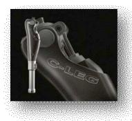
Microprocessor knee units utilize computerized mechanisms to evaluate the various stages of gait during a step and self-adjust to accommodate for speed and/or stability changes. Microprocessors are able to anticipate movement during a step and provide stable and seamless transitions between heel strike and toe-off.
