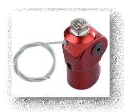
These knees are often referred to as 'stance control' knees and contain a weight-activated friction brake that stops the knee from bending. These knees swing freely, like a door hinge, when there is minimal or no weight put on the prosthesis. The knee locks once weight is applied. If the amputee attempts to put weight on the prosthesis when the prosthesis is partially bent, the weight-activated friction brake prevents the prosthesis from buckling.
